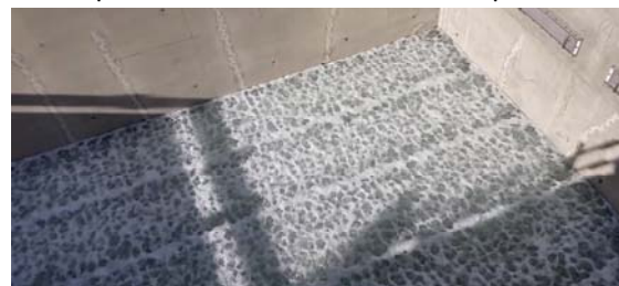
Carlsbad Filter Air Distribution Test
